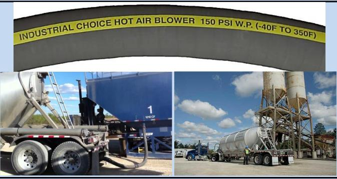
Designed for multiple applications where Hot Air up to 350°F is blown at PSI up to 1 150WPSI. Often used for bulk loading and unloading of dry material from plants and transport trailers. The hose is constructed so the tube won't dry out when air is pumped through it at up to 350°F. This hose will also pull a full suction/vacuum through it.
